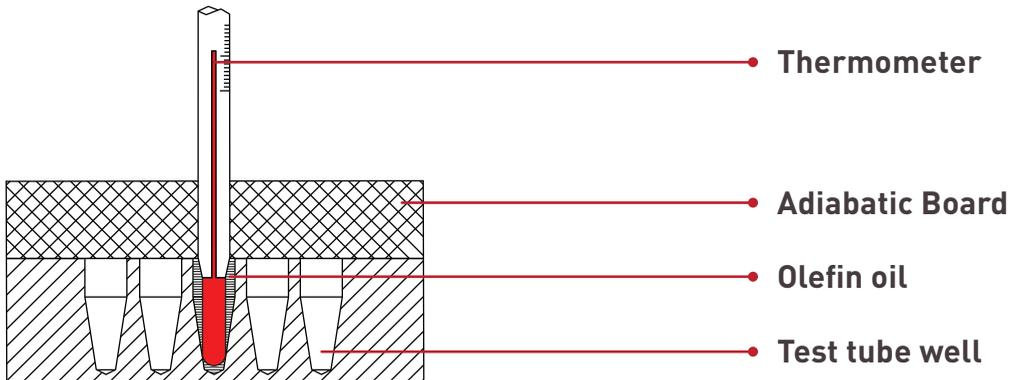
2. Press PGM's "▲" or "▼" in system setting interface, it will turn to Calibration, start calibration function. Then press Start/Stop key continuously, system will heat up to 40.0°C.
